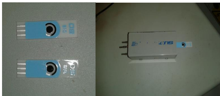
Fig. 2 Heavy metal sensors based on carbon –bismuth nanoparticles (a) and connecting box (b).
